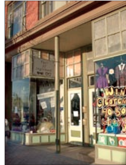
Large display windows, a clerestory of textured glass and large upper-floor windows on the Dougall Block contribute to a facade which substantially consists of glazed surfaces for a traditional brick structure. Other Ninth Avenue storefronts include glass bulkhead panels, an unusual feature intended to admit light into the basement storage areas.
